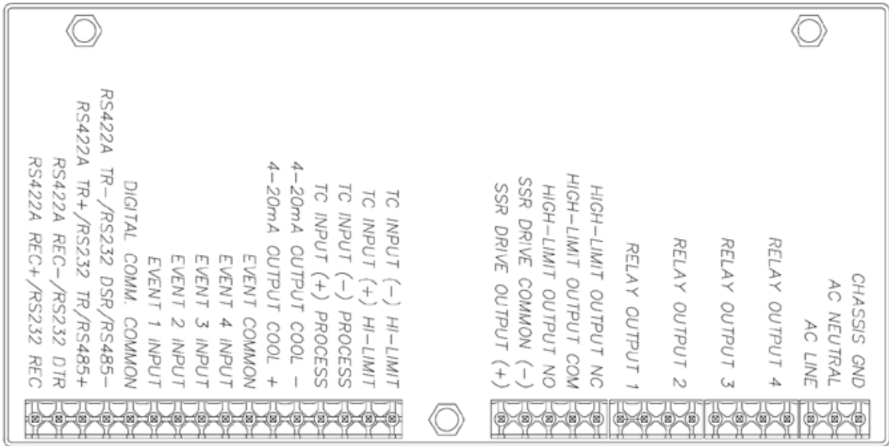
Figure 6. Protocol Plus Wiring Diagram.
