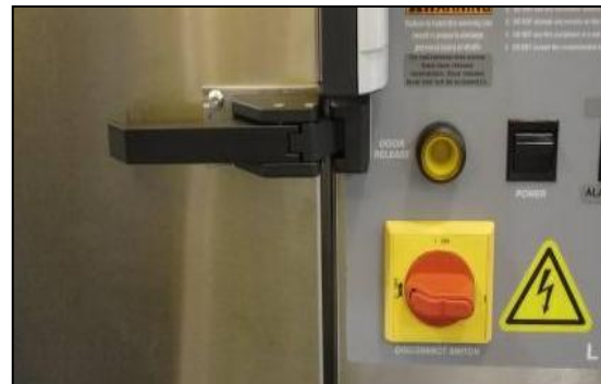
Figure 22. Door fully close and latch fully engaged.
