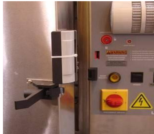
Figure 21. Oven door latch and door fully open (latch perpendicular to oven door).
