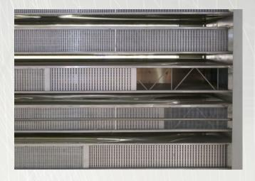
Novariance™ Technology provides extremely uniform airflow across the entire width of the tow-band and throughout the process chamber. Patent-pending orifice-plate nozzle structures eliminate the side-to-side and directional variance inherent in conventional nozzle designs. Airflow is also directed into the gap between the center supply plenums which eliminates an area of low to no airflow.
