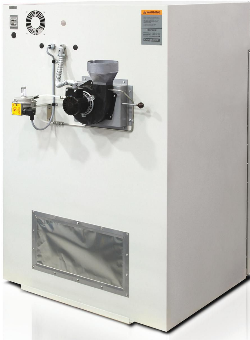
A foil relief panel may be preferred over explosion spring-latches or structural plugs on doors. The low mass of the foil panel reduces the risk of injury when it relieves.
