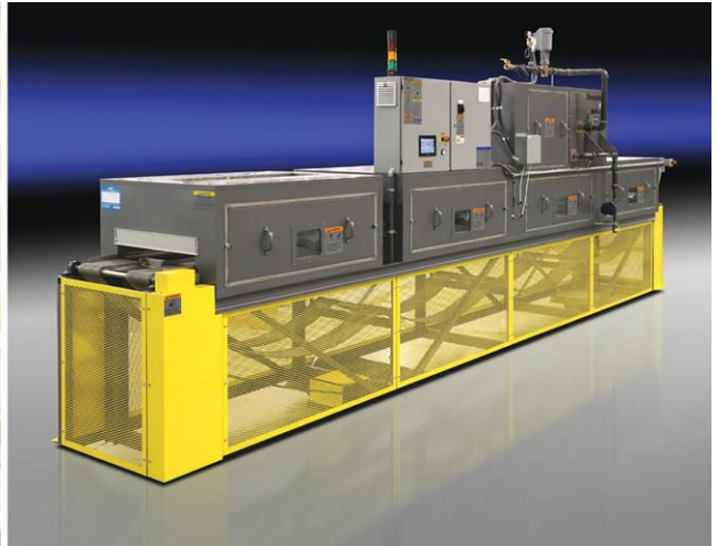
The drying solution for the bullet application was an oven that optimized airflow using perforated aluminum plates and a specially designed nozzle system. The dryer delivers both heat and airflow to the wet primer deep in the casing.
